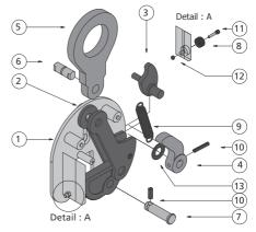
retaining pin (10) and take the lock assembly (3) out of the clamp.
