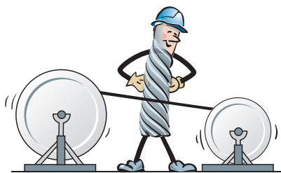
Figur 2-5 - do not create a reverse bend Figur 2-6 - Installing rope under tension, about 10% of the nominal rope pull
